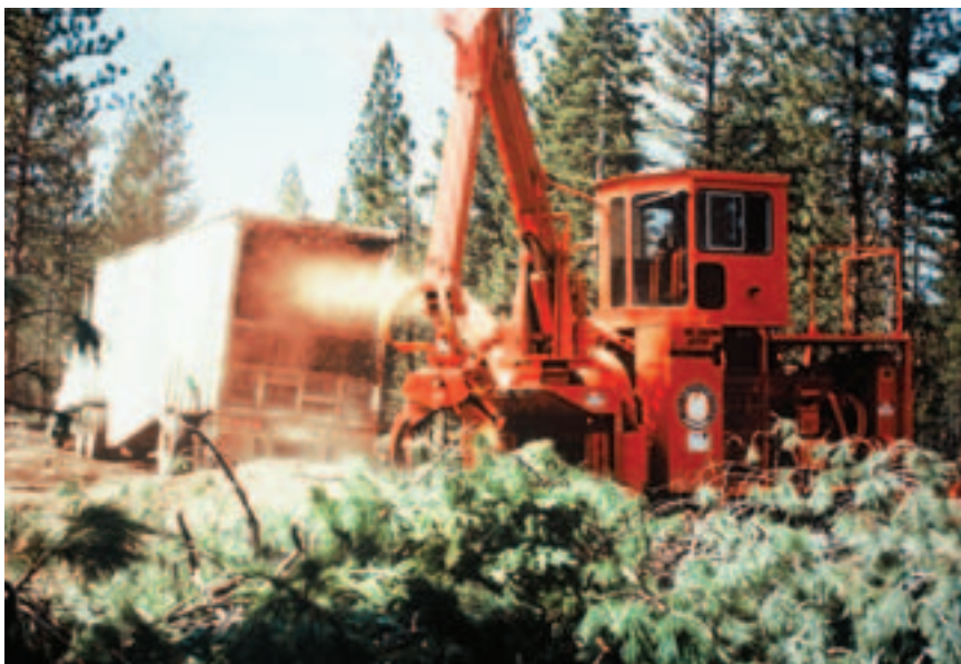
Biomass materials must be chipped in the forest and transported to biomass power plants. Each chip van contains enough fuel to power one home for about 250 hours.
