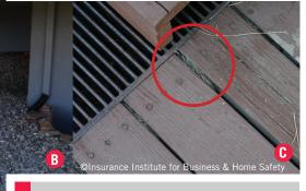
(A) Embers that pass through deck board gaps will land on the ground, or on combustible materials stored under the deck, as shown during this IBHS test.
