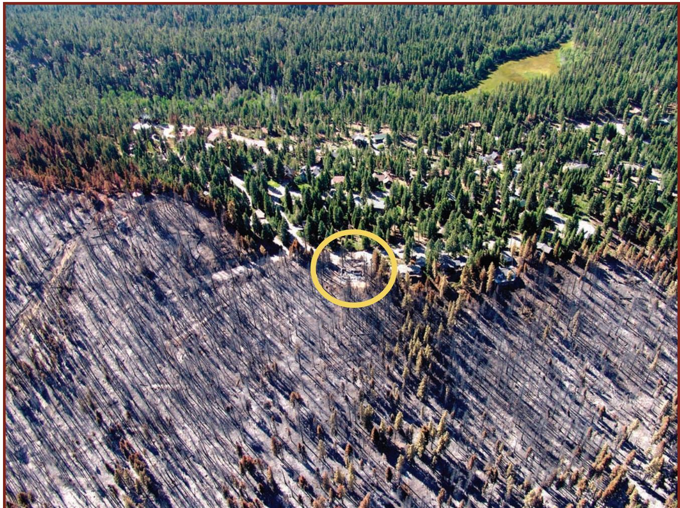
**Figure 6.** Single house which burned on Heather Circle in the Angora Highlands Subdivision. Note the location of house (yellow circle) on the edge of a steep slope exposed to an upslope crown fire run.
